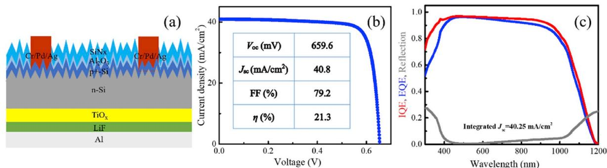
Fig. 3. (a) Schematic of n-c-Si cell with a full-area rear passivating, electron-selective  $\text{TiO}_x/\text{LiF}/\text{Al}$  contact. (b) Light  $J$ - $V$  curves under a standard AM1.5 g illumination and electrical parameters of cells with full area rear  $\text{TiO}_x/\text{LiF}/\text{Al}$  contact. (c) EQE, IQE and reflection of the cell.
