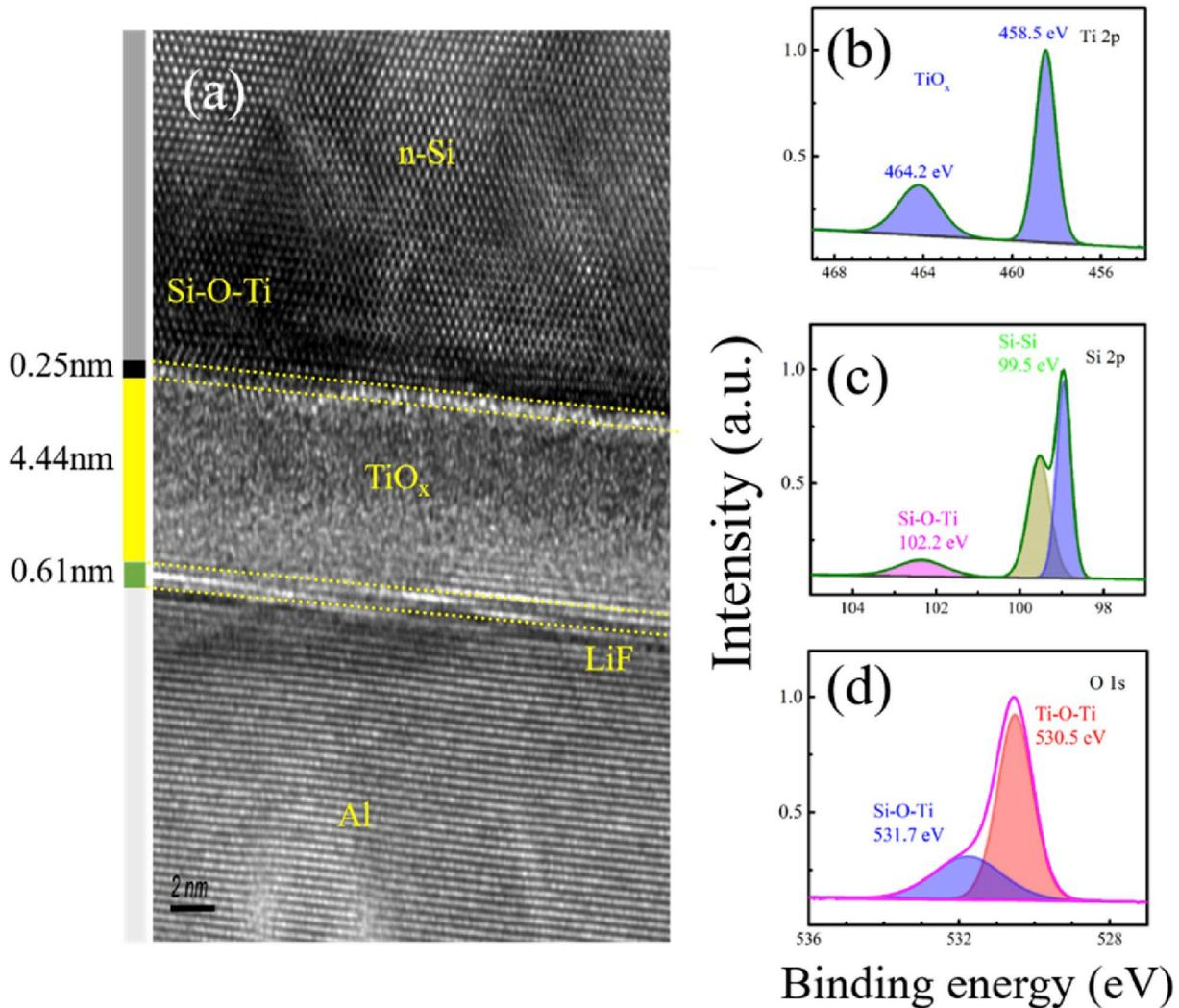
**Fig. 1.** (a) Cross-sectional TEM images of  $\text{TiO}_x/\text{LiF}/\text{Al}$  contact. Normalized X-ray photoelectron spectra of (b) Si (2p) (c) O (1s) and (d) Ti (2p) for  $\text{Si}/\text{TiO}_x$  interfaces with the  $\text{TiO}_x/\text{LiF}/\text{Al}$  contact.
