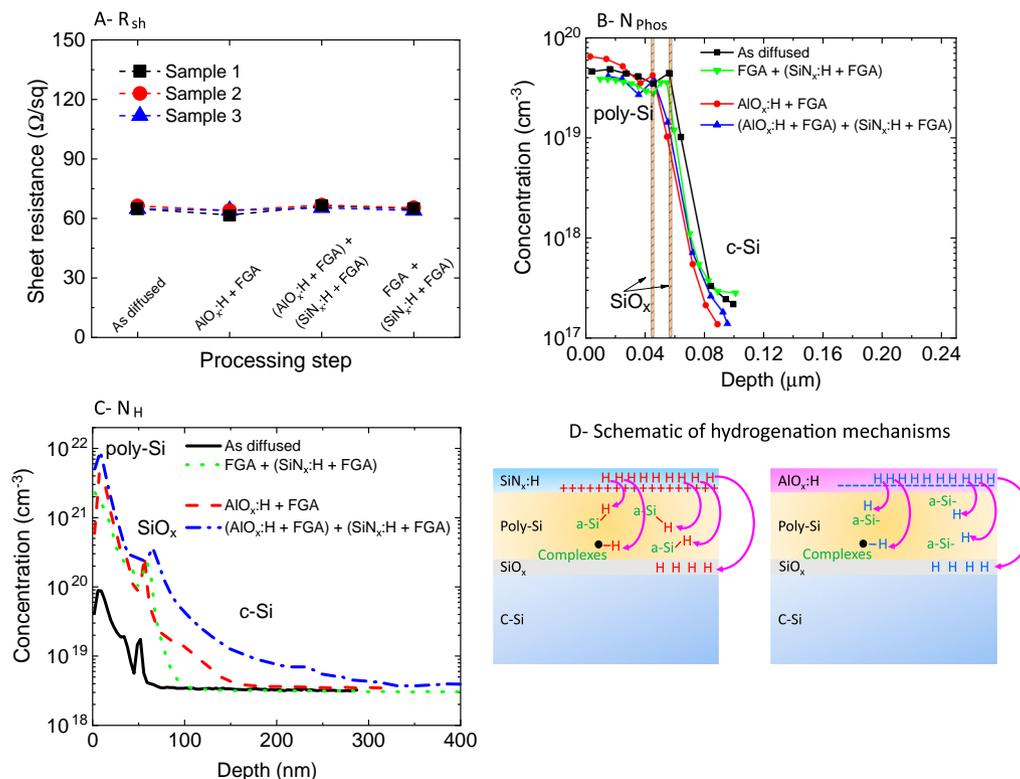
**Figure 4.** A) Sheet resistances of different samples at various processing steps. B) Electrically active phosphorus dopant concentrations by ECV measurements. C) Hydrogen profiles by SIMS before and after different hydrogenation steps. D) Schematic of the proposed hydrogenation mechanisms from different capping layers. The samples' substrate resistivity was 2 Ω cm. The AlO<sub>x</sub>:H films were deposited via the thermally assisted ALD technique.
