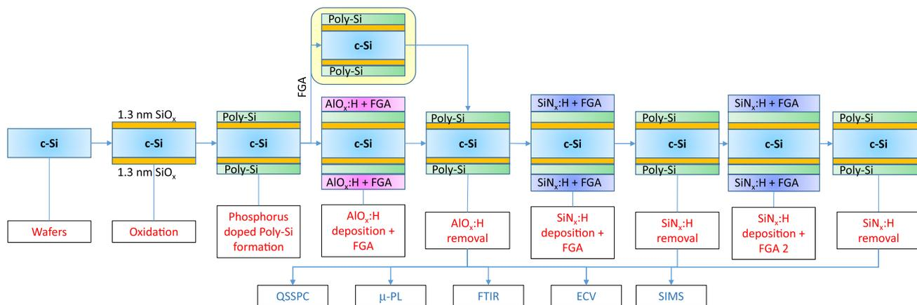
**Figure 2.** Schematic of the experimental processes.
