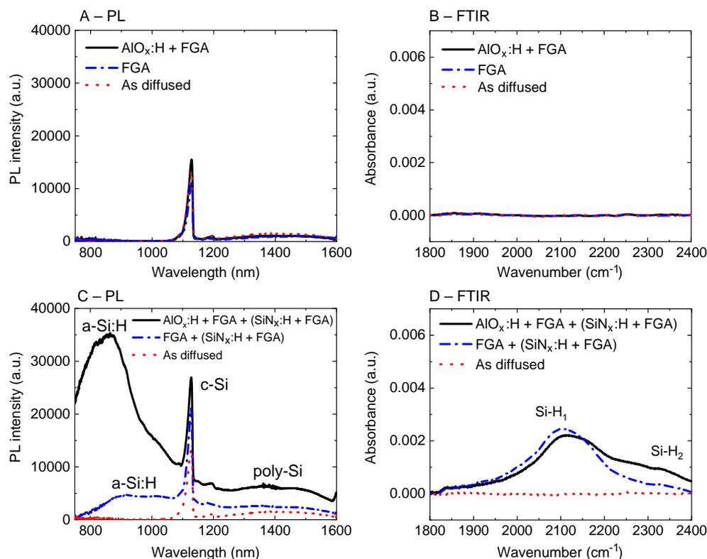
**Figure 3.** PL spectra captured from the phosphorus-doped poly-Si/SiO<sub>x</sub>/c-Si samples after A) plasma-assisted ALD AlO<sub>x</sub>:H + FGA hydrogenation and C) the subsequent SiN<sub>x</sub>:H + FGA hydrogenation, using the 405 nm excitation laser at 80 K. B,D) Their respective FTIR absorbance spectra in the Si—H wavenumber range of 1800–2400 cm<sup>-1</sup>. The samples' substrate resistivity is 2 Ω cm.
