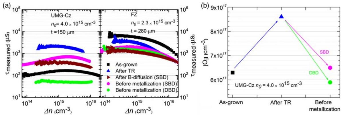
**Figure 1.** a) Injection-dependent minority carrier lifetimes of planar n-type UMG-Cz and FZ lifetime samples representing as-grown, after TR, after SBD, and after all high-temperature steps (before metallization) for both the SBD and DBD solar cell process, after etch-back and repassivation. b) Average  $[\text{O}_i]$  present in the UMG-Cz wafers measured by FTIR.
