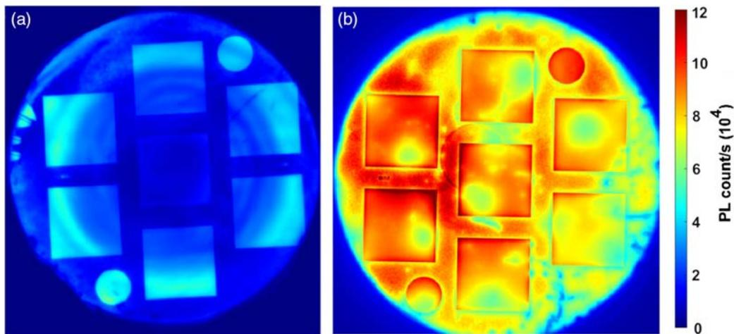
**Figure 2.** PL images of the 4-inch UMG-Cz cell precursors after all high-temperature steps (before metallization). a) DBD and b) SBD process. PL images were captured at an illumination intensity of 0.5 suns.
