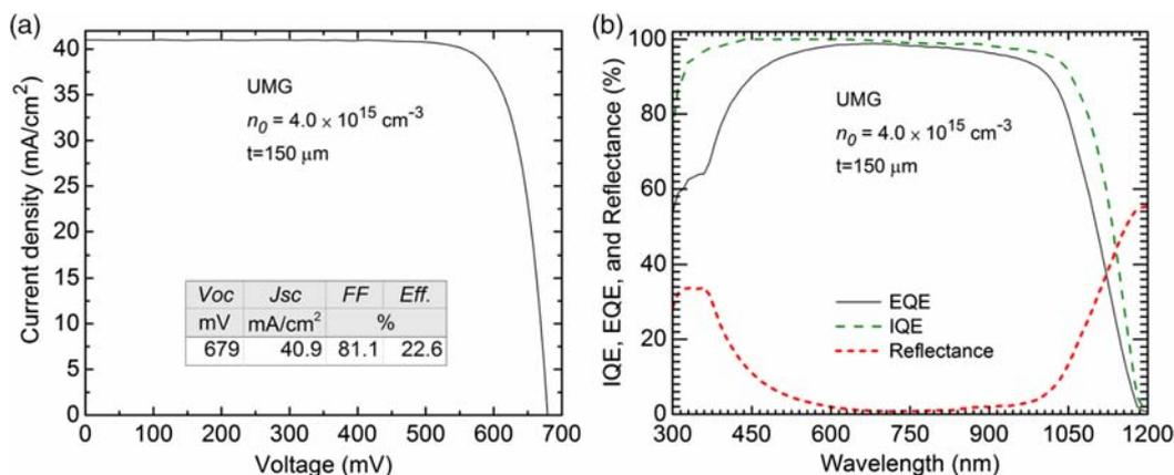
**Figure 3.** a) Measured  $J$ - $V$  curve for the champion UMG solar cell with homogeneous boron diffusion. b) Measured EQE, calculated IQE, and measured reflectance curves.
