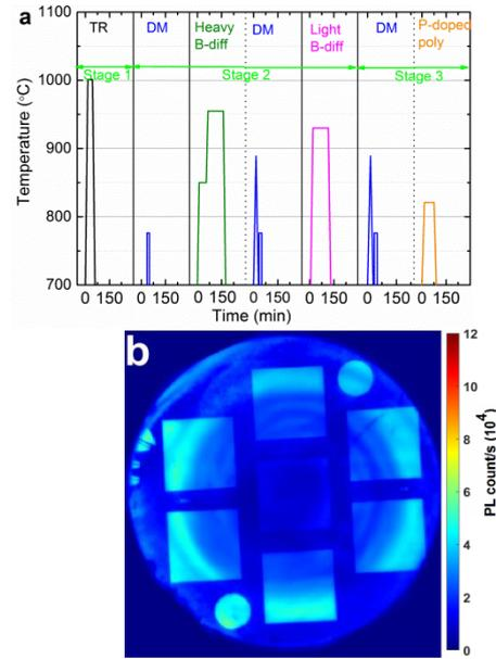
Fig. 4. (a) Thermal budget associated with the solar cell fabrication involving double-boron diffusion process. The duration indicates the total time that samples subjected to the given temperature. (b) PL images of the 4-inch TR-treated UMG-Cz wafers at stage 3 of DBD process. PL images were captured at an illumination intensity of 0.5 suns.
