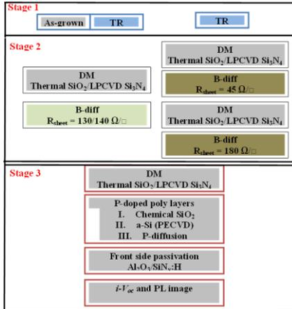
Fig. 1: Schematic of the solar cell fabrication processes used in this work.
