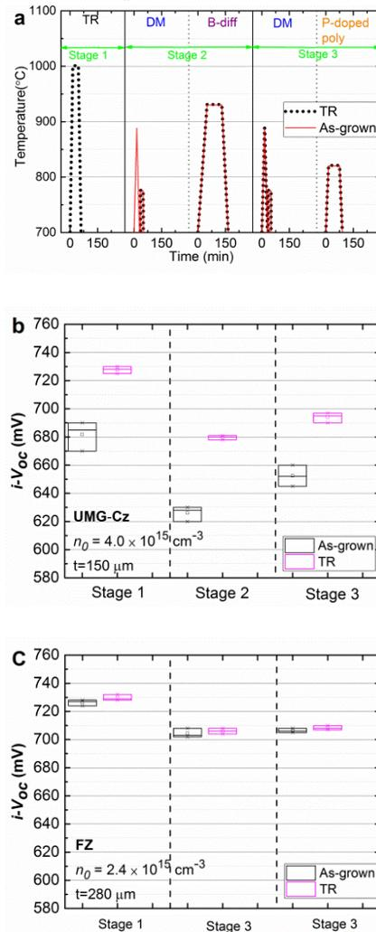
Fig. 2: (a) Thermal budget associated with the three stages of solar cell fabrication involving SBD process. The duration indicates the total time that samples
