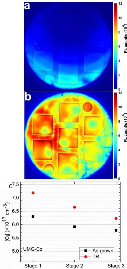
Fig. 3: PL images of the 4-inch UMG-Cz wafers at stage 3 of SBD process (a) as-grown and (b) TR-treated wafers. PL images were captured at an illumination intensity of 0.5 suns. (c) Average interstitial oxygen concentration measured by FTIR present in the UMG wafers after each stage, as shown in Fig. 1.
