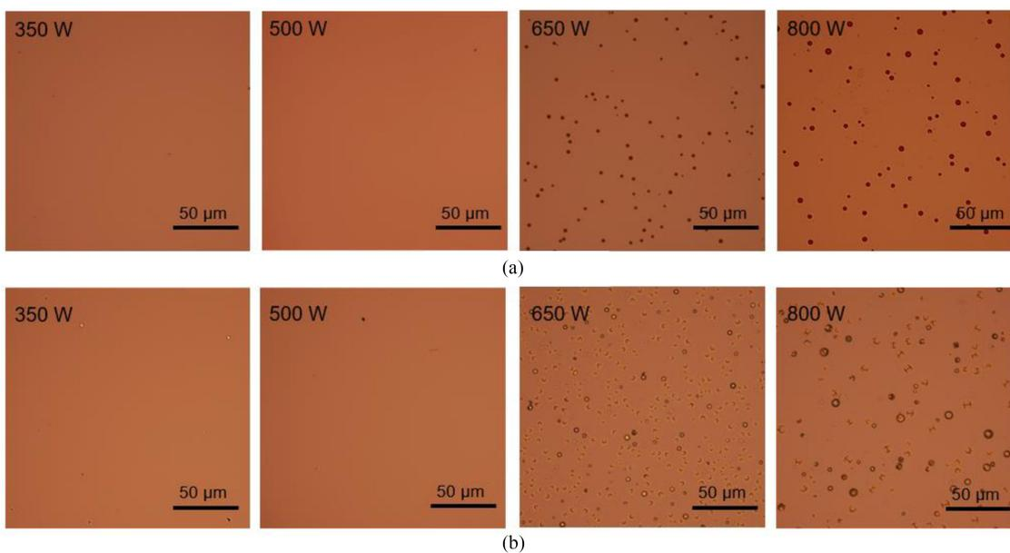
Fig. 2. Surface morphologies of (a) a-Si films and (b) doped-Si layers deposited by different PECVD deposition powers.
